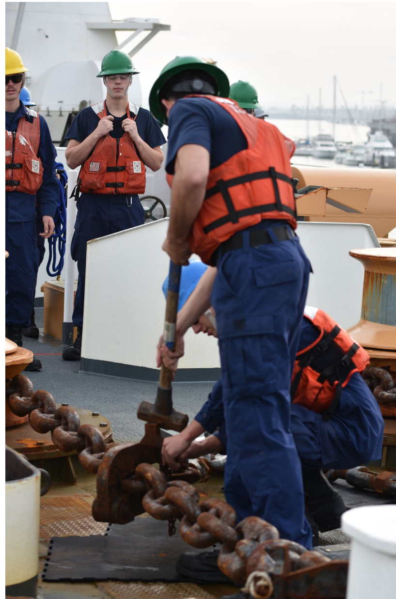
The MUNRO crew removing the pelican (chain stopper) as part of the anchor evolution so the anchor can be raised before departing from port.
