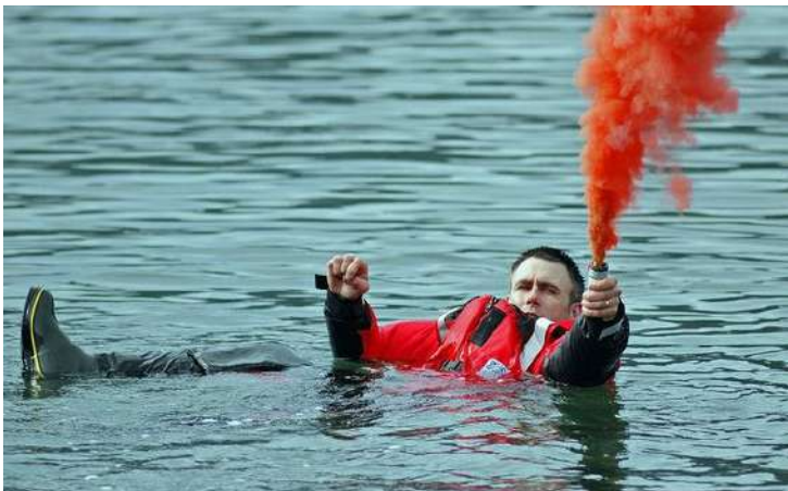
Handheld smoke signals, such as this one being tested by a Coast Guardsman, are highly effective attention-getters in the daytime.
