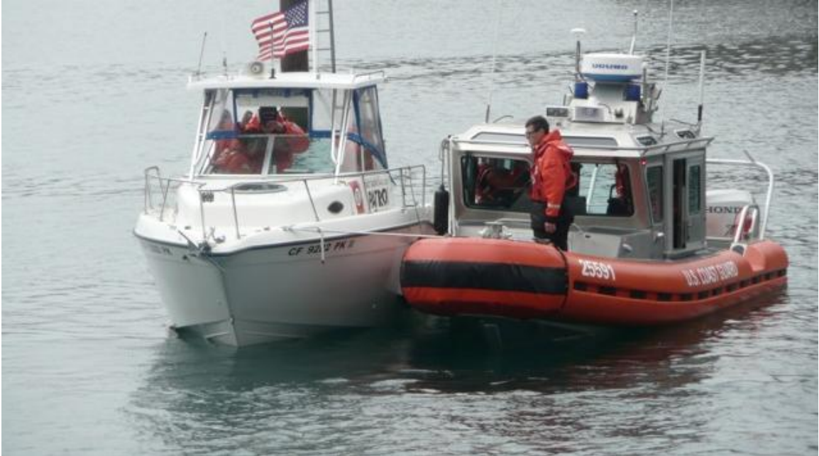
RBS 25591 with AUX Facility 179 in side tow
