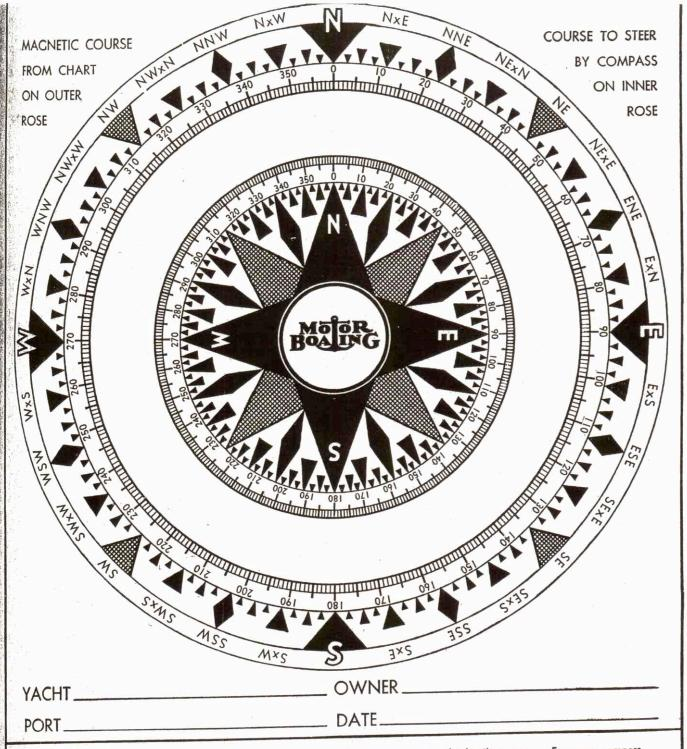
The OUTER rose represents MAGNETIC directions. The INNER card represents the boat's compass. For every compass heading for which the deviation is known, draw a line from that compass point or degree to the magnetic course (on the outer
