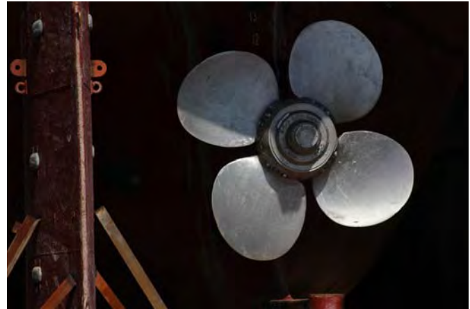
Nov. 9- The propeller of the tanker "Don Felix I" is exposed in dry dock in the Port of Tampa. To the left is the rudder which has been removed and temporarily tack welded in place.
