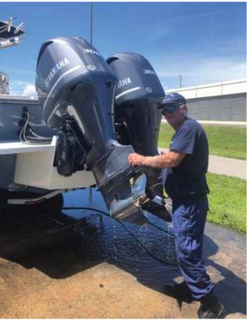
Above right: Steve Williams, member of Flotilla 74, Brandon flushes the saltwater out of the vessel's twin-engines after the Auxiliary patrol on Sept. 4. No doubt this image and the one above left are displays of our pride. USCG Auxiliary photos by George Papabeis
