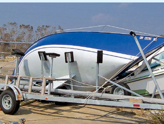
Most boats do well on trailers in a hurricane. The exception is deep-draft sailboats, which are vulnerable when the wind is on the beam. Whenever a sailboat with a deep keel is stored on a trailer, jack stands should be used to provide additional support.
