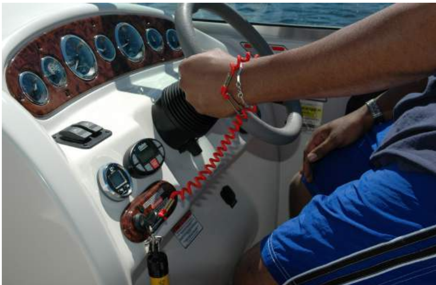
An emergency cut-off lanyard is an important piece of safety gear that all boat operators should wear in case of falling overboard.
