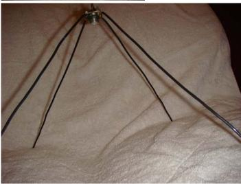
The SO-239 coaxial connector is the basis for the antenna. If you can get a silver plated connector it will be easy to solder the ground plane wires to it after you put in the #4 brass machine screws to hold the ground plane wires in place. If the connector is plated with some other material don't try to solder it (except for the center conductor, which must be soldered in place.)
