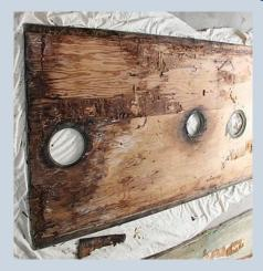
The Melroy's deck plate had dry rot and had to be replaced. After 20 years of service, the deck felt soft to walk on and after removal, it was clear why this was so. This photo shows the rotted deck plate after removal from the boat.
