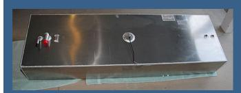
One of the biggest issues facing our flotilla was replacement of the old fuel tank. The old tank had considerable corrosion and prior to replacing the engines, we felt it would be wise to replace the tank.
