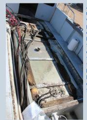
After the deck plate was removed, the next step was removal of all of the polyurethane foam around the tank. This foam had to be removed so that the tank could be extracted. "Foaming" fuel tanks was popular at one time but now has been largely discontinued because of crevice corrosion associated with this method.
