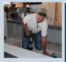
Once the T Top and center console were removed it was time to extract the original fuel tank. This tank had old fuel in it and was corroded after twenty five years of service. Here, John Boyne removes all of the deck plate screws in preparation for fuel tank removal.
