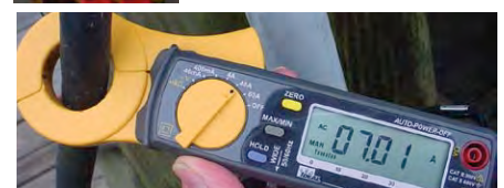
Top: An inexpensive circuit tester. Bottom: This clamp meter shows a 7-amp difference between the current going into the boat and coming out.
