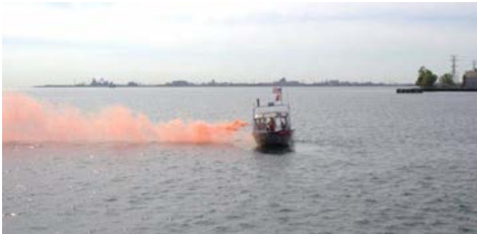
Facility NU-SAR demonstrates a hand-held orange smoke flare. All of the orange powder drifted downwind and stayed off the boat.
