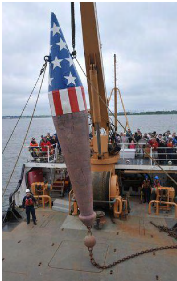
BALTIMORE - The Coast Guard Cutter James Rankin, a 175-foot buoy tender homeported in Baltimore, lifts the Francis Scott Key buoy off the deck in order to lower it to its location in the Patapsco River, May 24, 2010.
