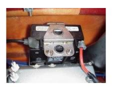
kill switch mechanism must be in proper working order. All PWCs require an operating self circling or kill switch mechanism.
