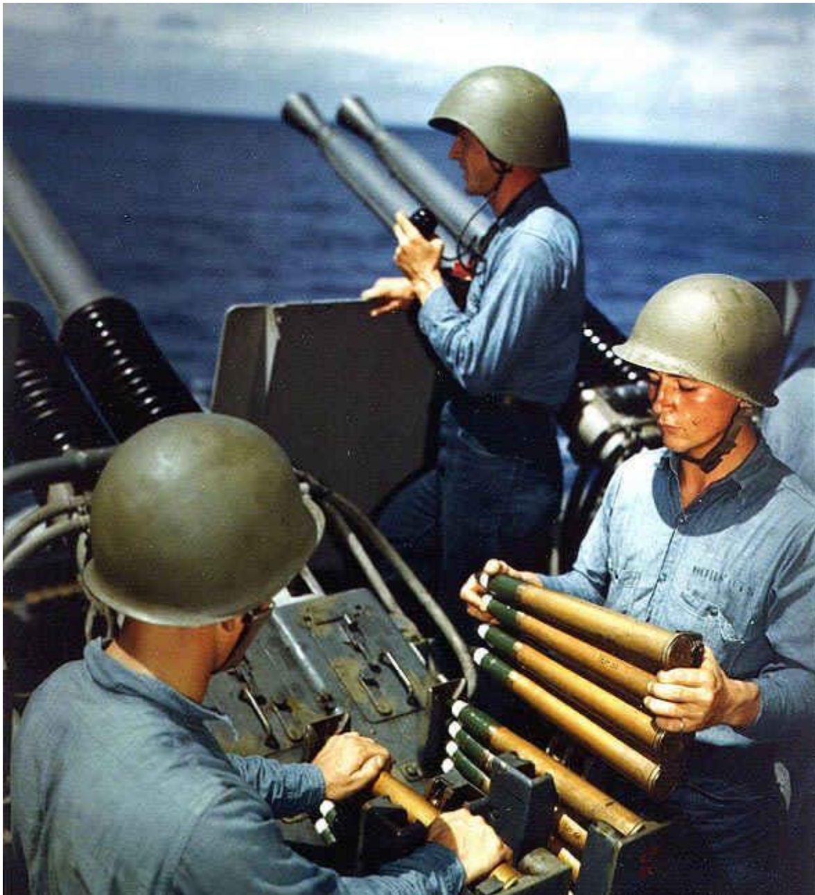
Crewmen feeding four-round HE-T/SD [40 mm] ammunition clips on USS Alaska CB-1 in 1945. U.S. Naval Historical Center
